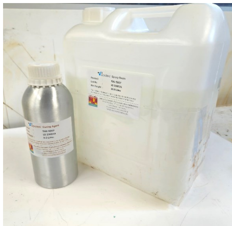
Figure 3-5: Two-part Recyclamine-based Epotec YDL_5557/THR 9357.
