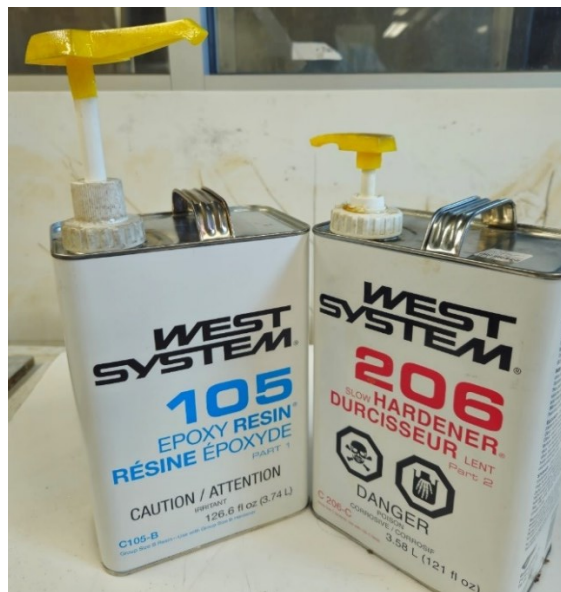
Figure 3-6: Two-part West System 105 Epoxy Resin and 206 Hardener.
