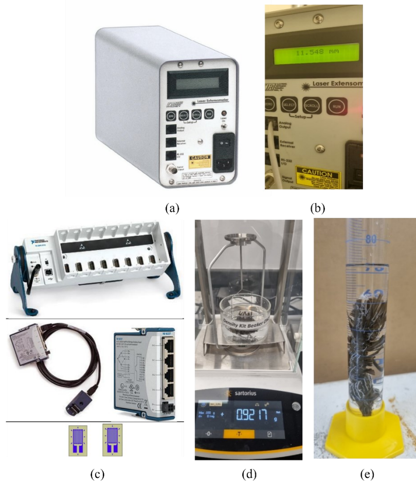
Figure 4-2: (a) and (b) the laser extensometer, (c) NIDAQ data acquisition system, (d) the balance, (e) the graduated cylinder.
