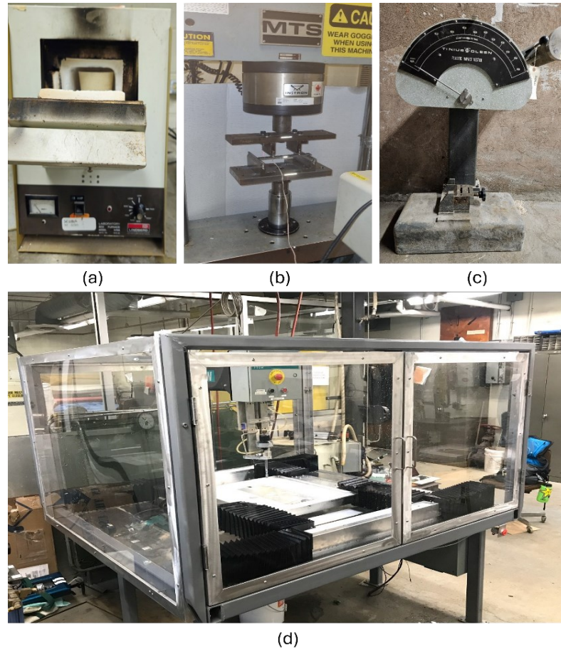
Figure 4-1: (a) Muffle Furnace, (b) MTS Universal Testing Machine, (c) Izod Impact Tester, and (d) Waterjet Cutter.
