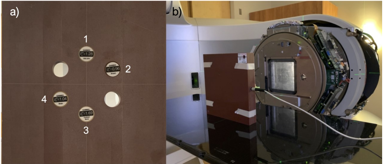
Figure 19. a) In-house contrast phantom containing 1) CB2-30% 2) breast 3) cortical bone 4) brain tissue equivalent inserts and two voids for additional materials and b) thin contrast phantom imaging setup at 98 cm SSD.
