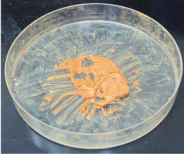
Figure 3.1. Millbase (Binder/linseed oil and pigment/henna) paste was created to be combined with a solvent (propylene carbonate) for the desired consistency.
