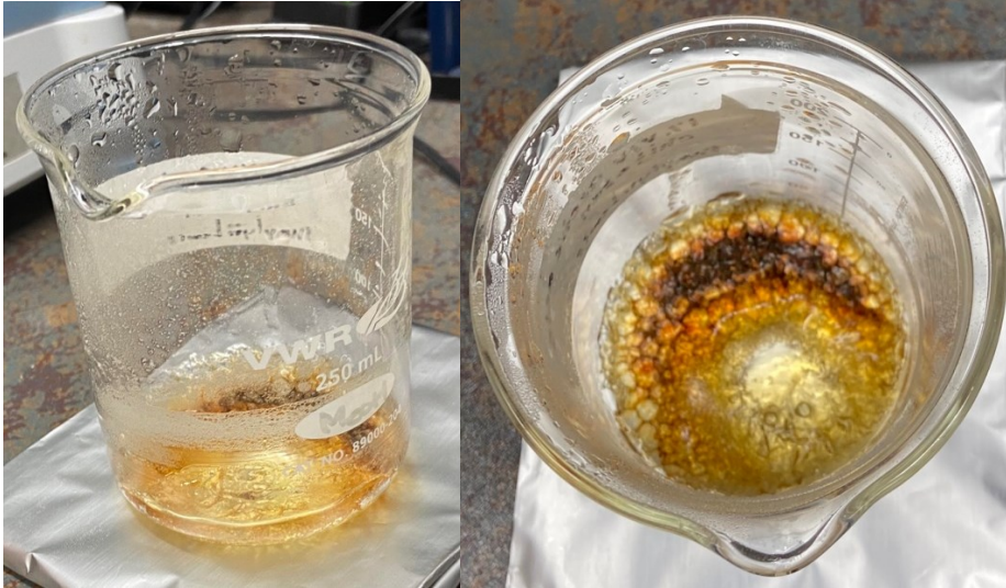
Figure 3.3. First trial synthesising chitosan nanoparticles from chitosan. Trial was over heated and burned, sticking to the glass beaker resulting in an unusable test trial methods were adjusted following this trial. Side (left) and aerial view (right)
