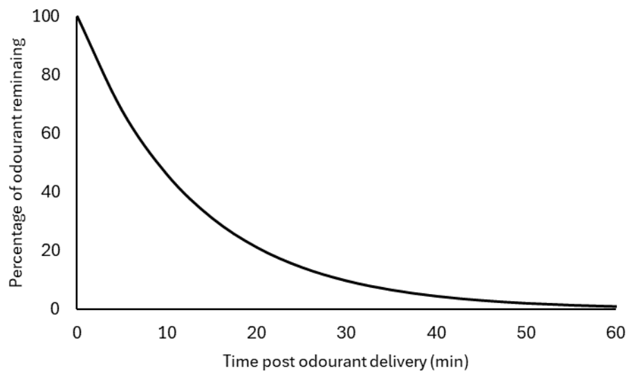
Figure 21: Theoretical calculation of odourant dilution after delivery to the tank based on water flow.
