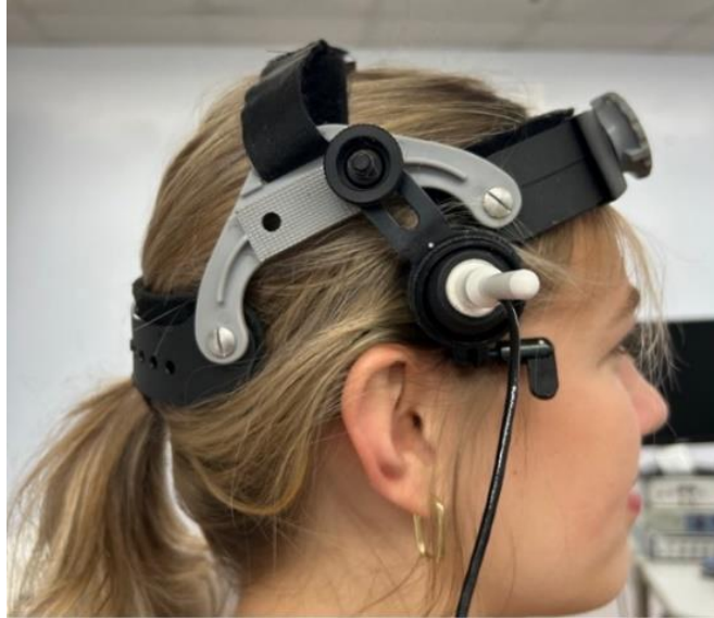
Figure 3.1. Schematic view of the transcranial Doppler 2-MHz probe over the trans-temporal window, secured with a custom headset.
