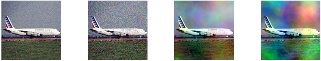
(a) AWGN with \sigma = 0.3 (far left) and \sigma = 0.6 (left). Brownian noise with \sigma = 40 (right) and \sigma = 70 (far right).
