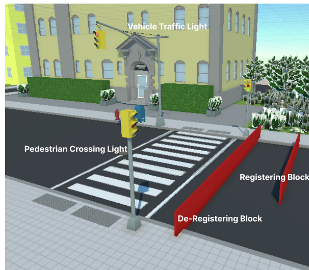
Figure 3.10: Components of the Traffic Controller System deployed at each crossing in the map
