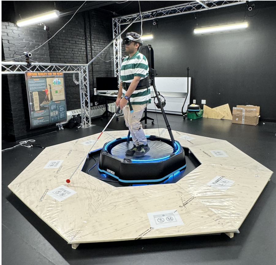
Figure 4.3: Slide mill setup with the wooden skirt
