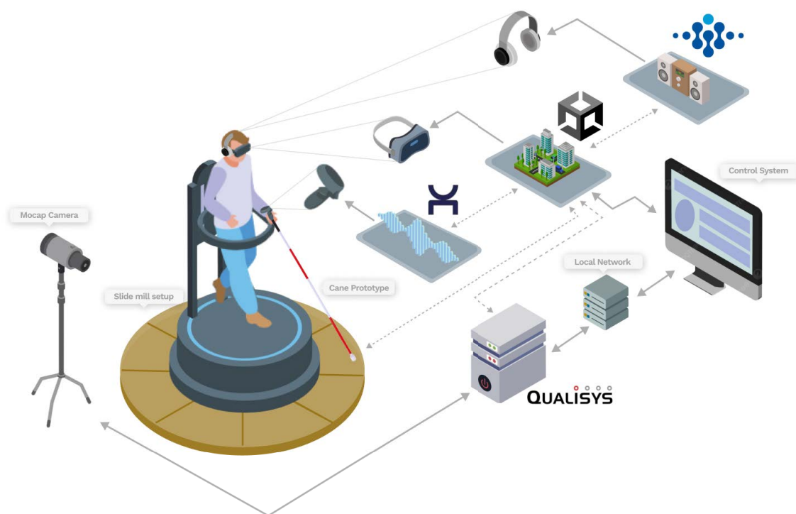
Figure 3.4: High-level system architecture: A broad overview showing key components and their interactions
