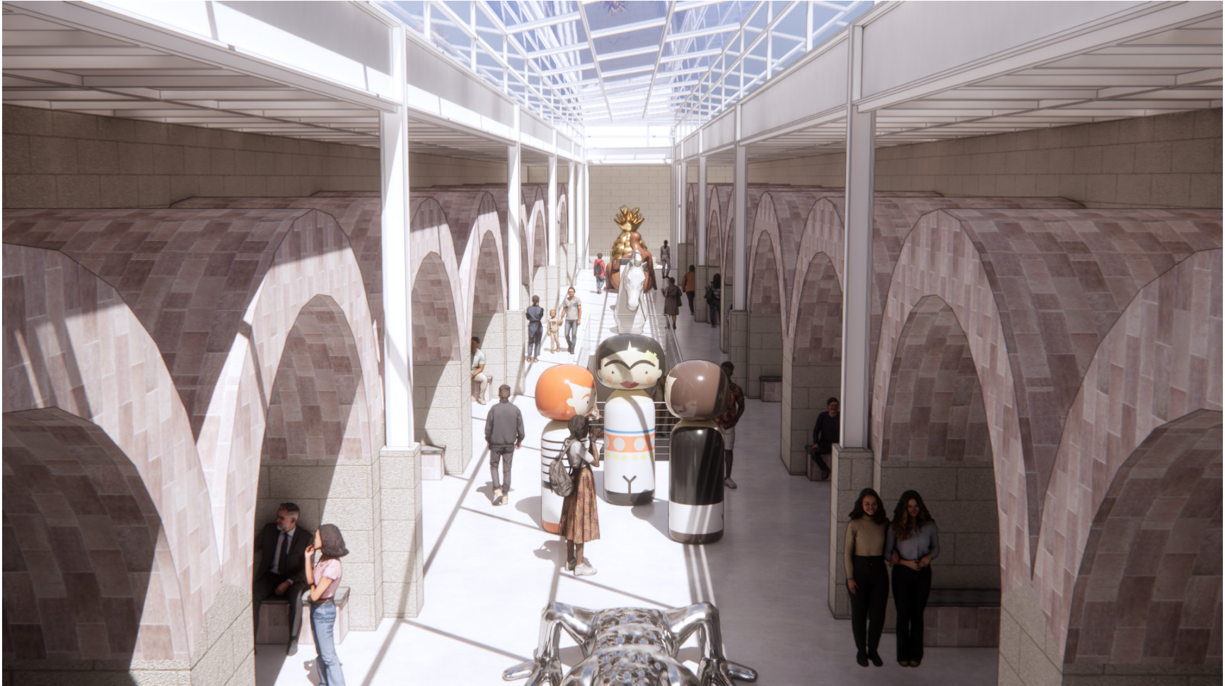
Figure 78: Render image of Parade level of Museum Galleries - the upper floor of the museum galleries are flooded with natural light from the sky roof above. Casemates offer protection from UV damage to items on display and have benches built along their edge to rest and engage with the exhibits.
