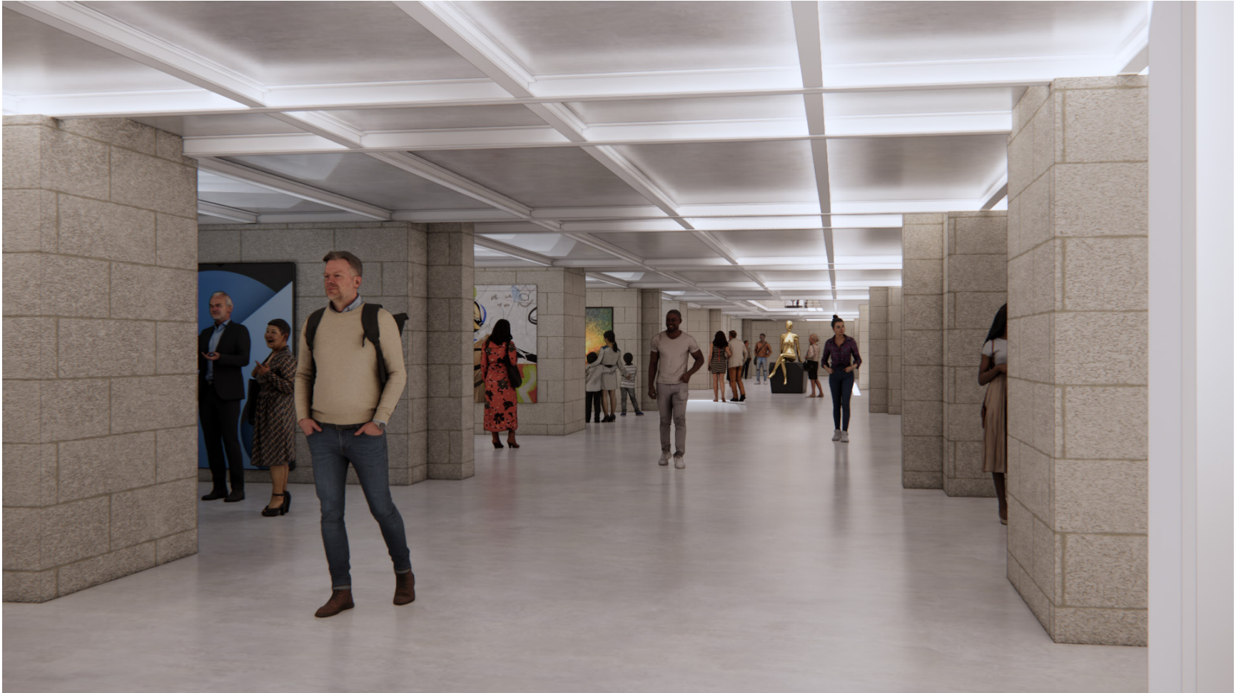
Figure 79: Render image of Museum Galleries Lower level - The lower level galleries have partial natural light fed through central voids in the upper gallery floor. The lower level galleries primary lighting is pocketed in the upper flange of the flooring grid serving the upper level. This provides a consistent bathing of ambient light suitable for displaying UV sensitive and precious exhibits.
