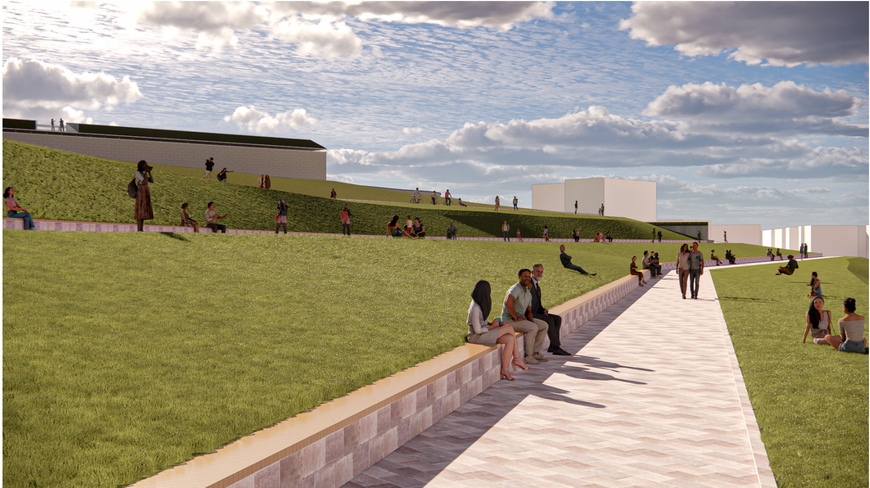
Figure 33. Rendered image of Glacis pathway along the Ring Path Network. Each pathway follows a single contour allowing for barrier-free perambulation of the city and a 360 degree view of Halifax. The benches line the upper edge of each path are made from masonry removed from the Fort George casemates.
