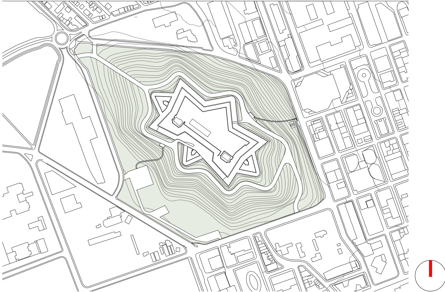
Figure 21. Plan drawing of the Citadel National Historic Site with the Glacis highlighted in green
