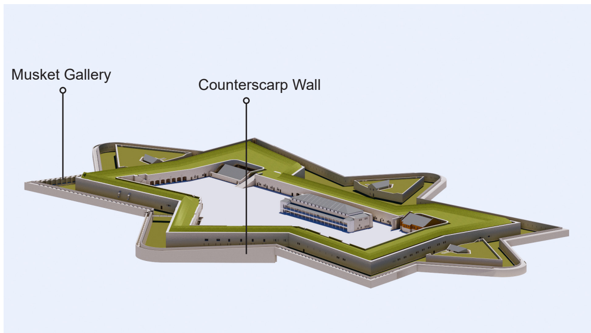
Figure 14. The Counterscarp wall surrounds the ditch dropping from the crest of the Glacis 40' - 45' below. Within the Counterscarp wall is an tunnel system surrounding the fort known as a Musket Gallery. The Musket gallery serves both as a full perimeter circulation and defence - the wall is perforated with rifle slots.
