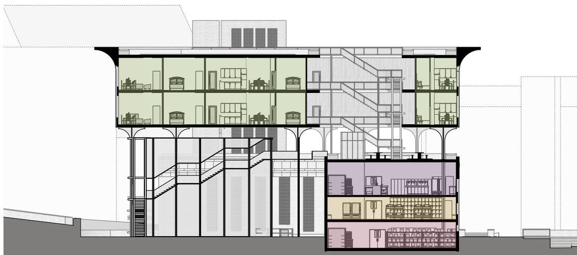
Site section depicting the residential units highlighted in green, and the kitchens in purple, the shelter in yellow, and the donation and distribution center in pink.
