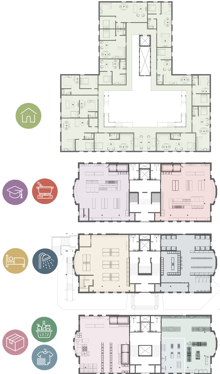
Floor plans depicting the residential units highlighted in green, and the training kitchen in purple, the commercial kitchen in red, the shelter in yellow, the bathing facilities in blue, and the donation and distribution center in pink, green and light blue.
