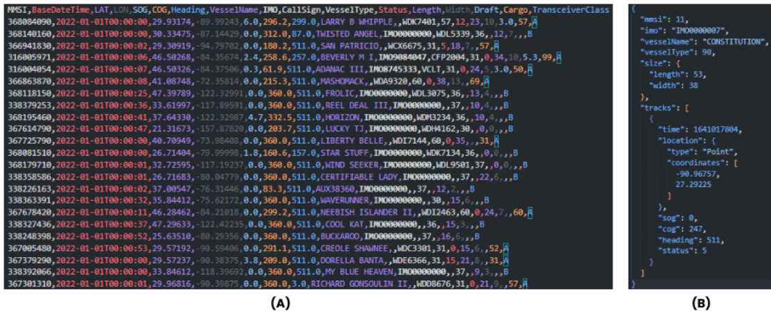
Figure 3.5: AIS Data structure A) Raw data AIS data from CSV B) preprocessed AIS data
