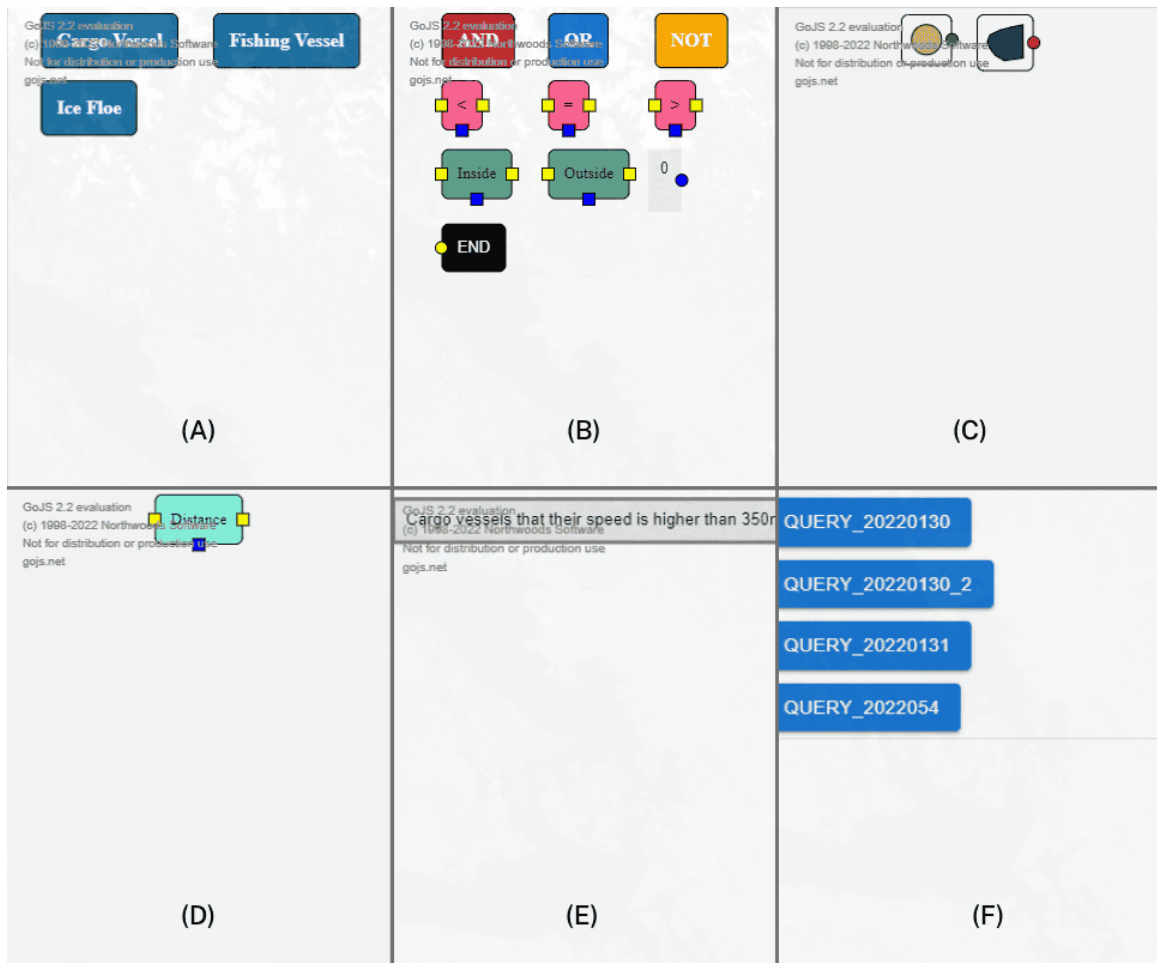
Figure 3.12: Visual query builder palette, A) Entity nodes B) Conditional nodes C) Selection Nodes (User selections over the map) D) Functional nodes E) Template nodes F) Query history
