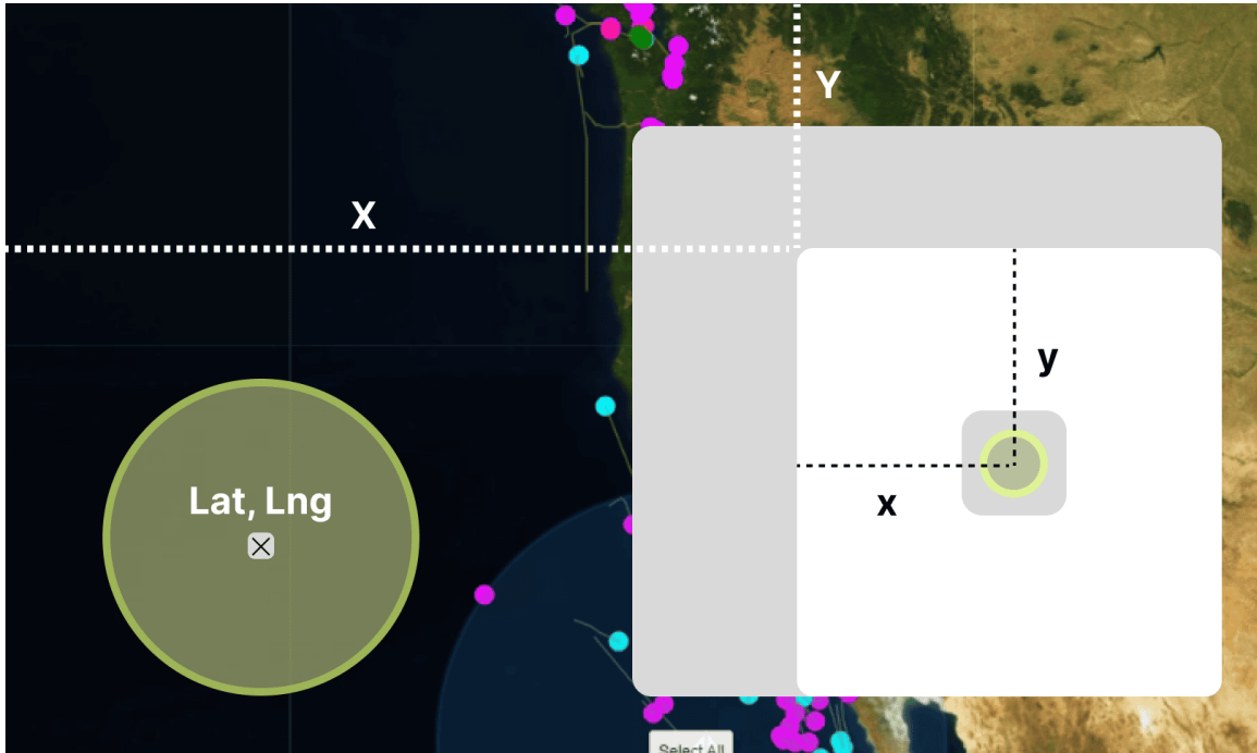
Figure 4.3: Determining the arch's initial and terminal points: X , Y represent the absolute position of the workspace relative to the tabletop's origin; x , y indicate the selection node's relative position within the workspace; lat, lng denote the geospatial coordinates of the center of the selection (highlighted as the yellow circle in this figure).
