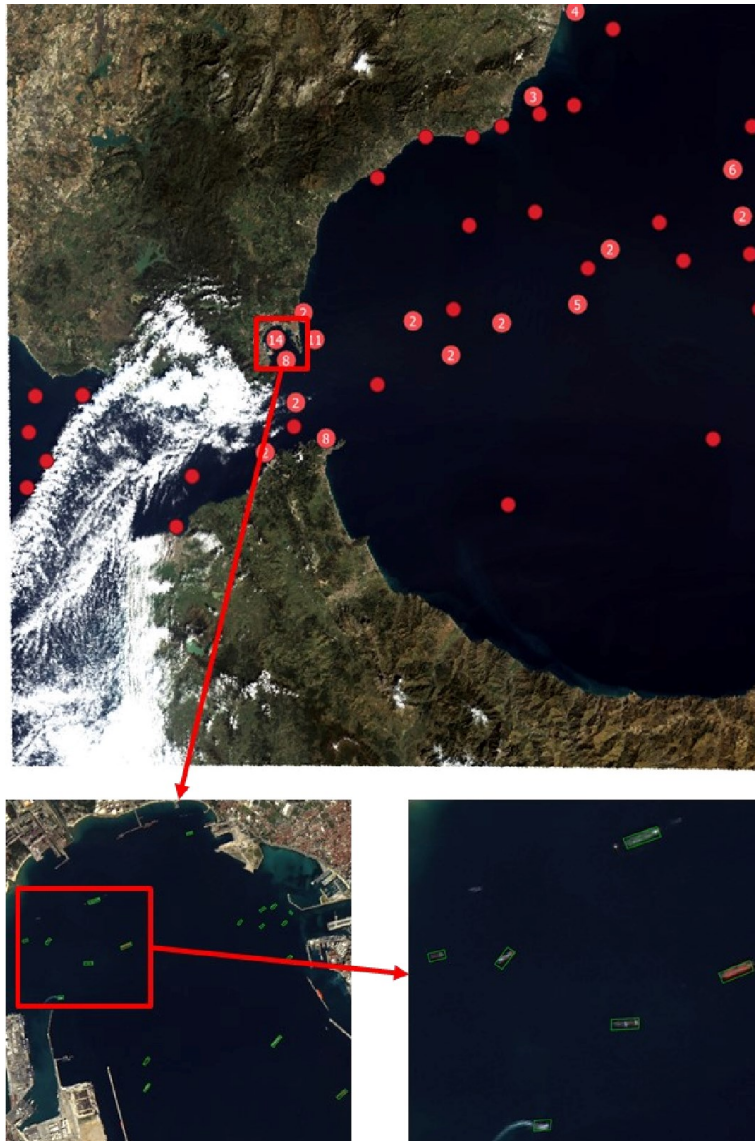
Figure 5 Example of medium resolution (Landsat-8) optical image ML vessel detection results [26]. 62% of vessels 30m or longer were detected using 15 m GSD imagery using the RGB trained model. This was considered suitable for suitable as a tool for sea traffic monitoring.
