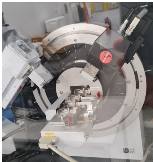
Figure 19 Bruker D8 Advance X-ray diffractometer with X-ray emitter (left), detector (right) and eight sample rotatable stage
