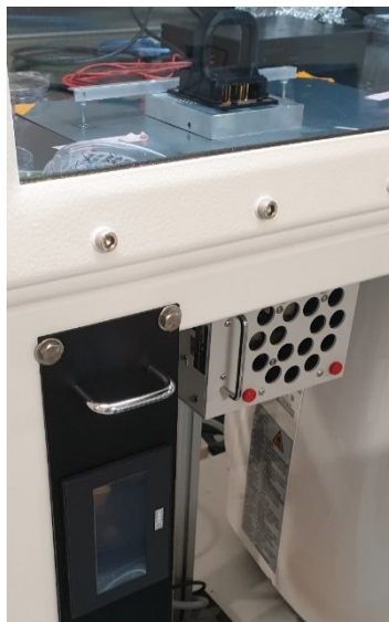
Figure 25 Solar cell testing apparatus with solar simulator mounted below the glovebox and solar cell mounting plate and contacts inside glove box
