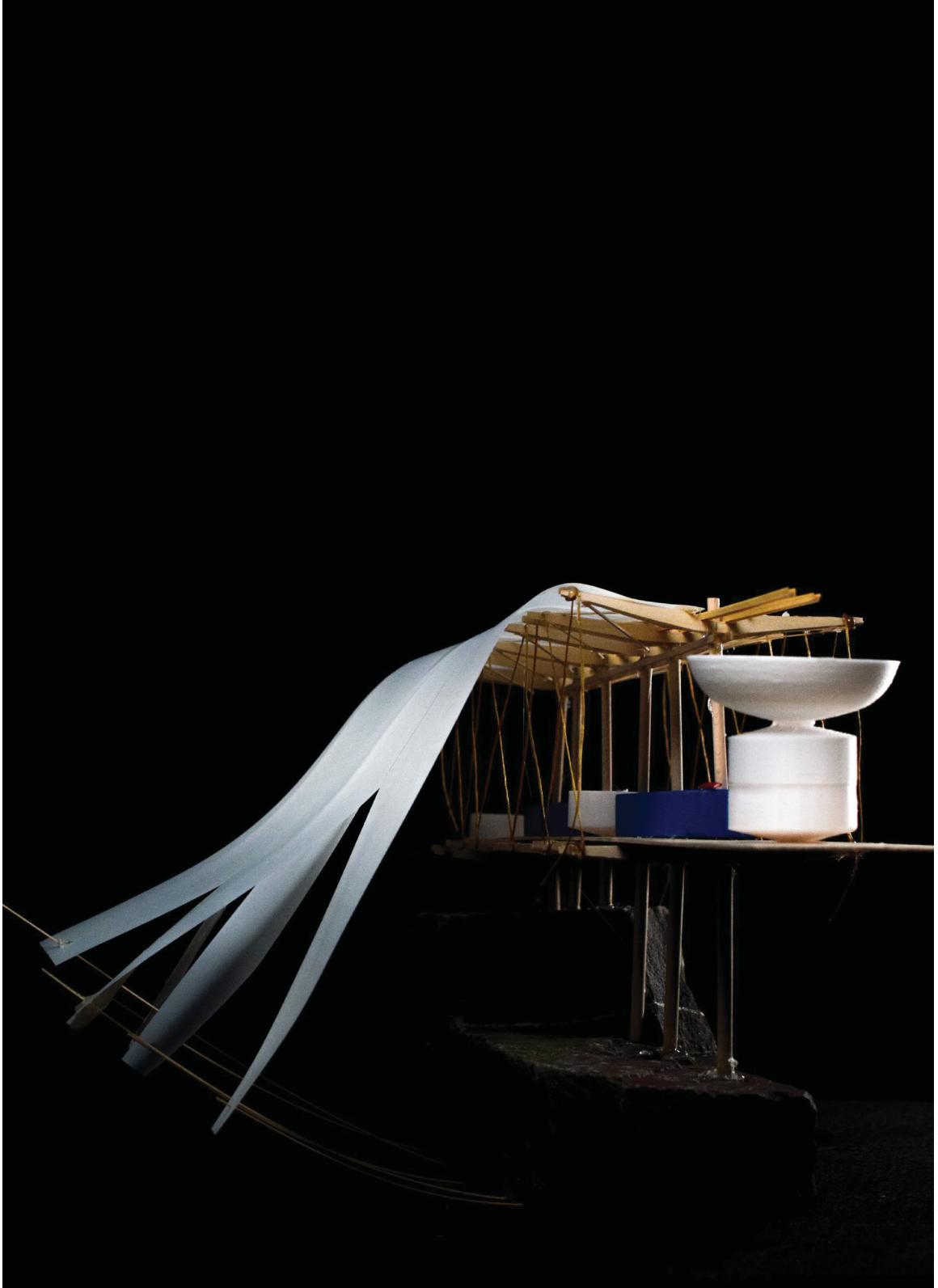
Sketch of the gumbo house , showing the built-in gutter sitting on the recessed part of the butterfly roof; the granite base is a found-object from Horton Landing, NS.
