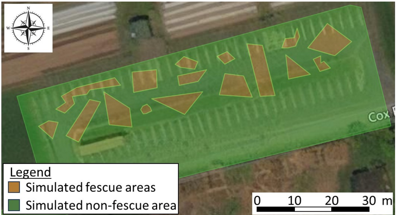
Figure 4-4: Prescription map of parking lot at Dalhousie Agricultural Campus, Bible Hill, Nova Scotia, Canada with arbitrarily drawn polygons for lab evaluating the applicators control and actuation systems. The green polygon simulates the non-fescue areas and the orange polygons simulate the fescue areas.
