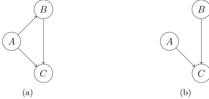
Figure 2.1: The graph representing the causal structure of the SCM considered in section 2.2.1, with three variables A, B , and C with the causal relationships A \rightarrow B, A \rightarrow C , and B \rightarrow C . The graph is shown both (a) before an intervention is performed and (b) after an intervention do(B = b) has removed the causal relationship A \rightarrow B .
