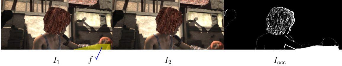
Figure 2.5: Example of occlusion: the occlusion mask is shown in I_{occ} with white pixels being the occluded ones. The yellow region in I_1 becomes occluded as it moves out of the scope of the image in the direction of f which resulted in having no matching pixels in I_2 .
