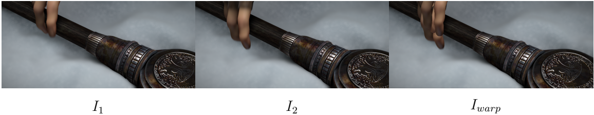
Figure 2.6: The repeated pattern occurs in I_{warp} as I_2 is backwarped to I_1 following the optical flow f_{1 \rightarrow 2}
