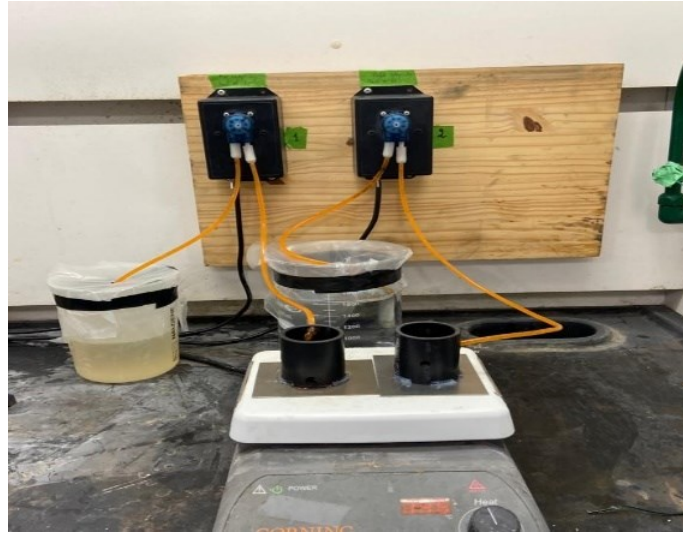
Figure 15 - Test coupons are placed on a hot plate and supplied with fluid using a peristaltic pump.
