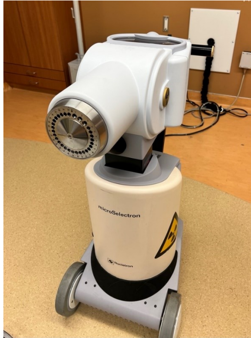
Figure 1.4 The remote afterloader used at the QEII Cancer Centre in Halifax, NS
