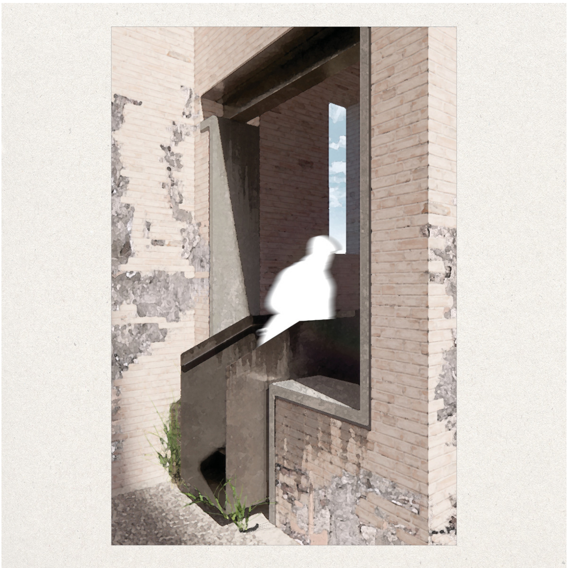
Top of the spiral staircase. The steel stair extrudes into a path, dropping visitors off onto the second floor of the Powerhouse. A new I-beam above supports the new opening.
