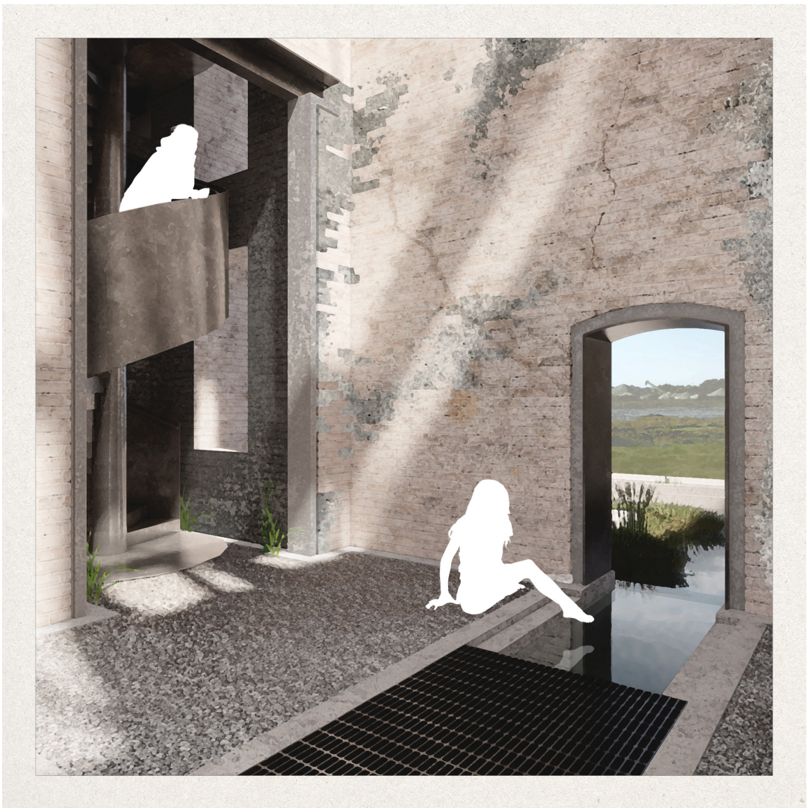
Base of the spiral staircase. Human and water circulation here cross over and creates a space to observe peculiar imperfections in the brick. An incision lets water and a view out to the harbour.
