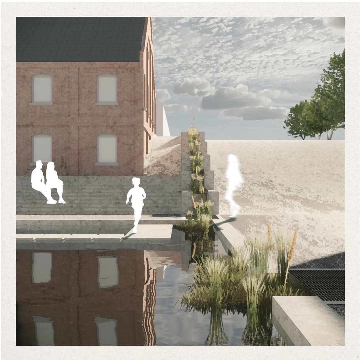
Path facing back into downtown Victoria. A series of terracing bioswales planted with sedges and catstails clean stormwater and collect it into the Plaza.
