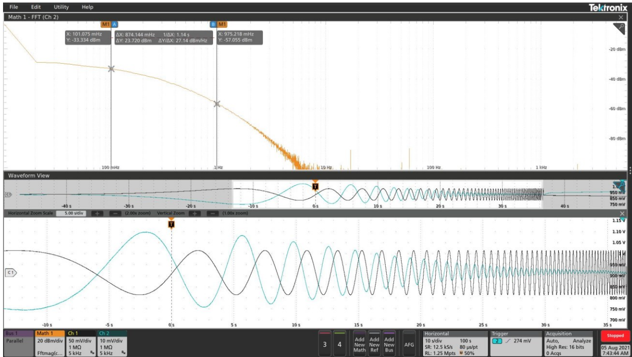
Figure 66: One example of the filter response for the low pass filter using a chirp signal.
