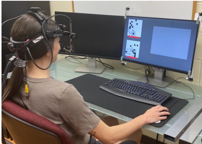
Figure 5. The experimental set up. The primary monitor displays the simulation. Although the monitor on the left does not display anything while the simulation is running, planning exercises as well as SA and workload measures were completed on this adjacent monitor.
