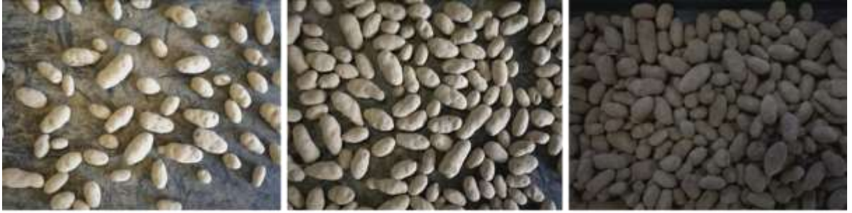
(a) (b) (c) Figure 3.2: Images of the tubers acquired on laboratory conveyor belts showing (a) sparse clustering, (b) moderate clustering, and (c) dense clustering scenarios.
