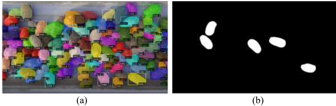
Figure 3.8: Densely clustered image in a cloudy scenario showing (a) tuber segmented image and (b) 5 fully visible tubers sampled from those detected.
