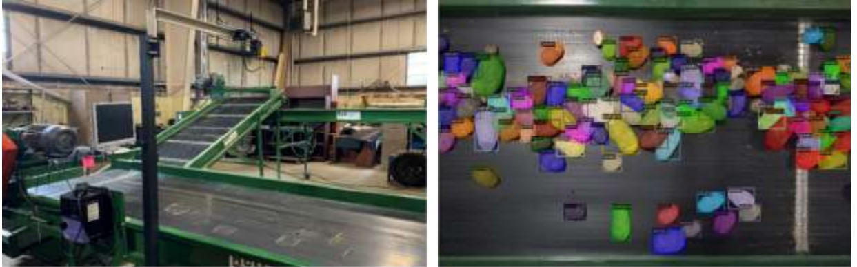
(a) (b) Figure B-1: (a) Laboratory set-up for image acquisition and (b) annotated image sample of tubers on the laboratory conveyor (section 3.2.2)
