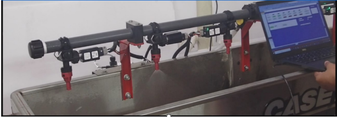
Figure 3.2: Testing the laptop nozzle control software opening Nozzle 2 (Second from left) of the static sprayer.
