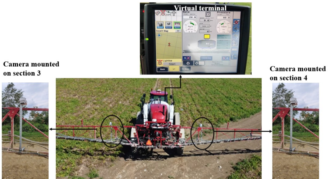
Figure 5.4: Cameras of outdoor MVS mounted on CASE IH Patriot 3340 sprayer.
