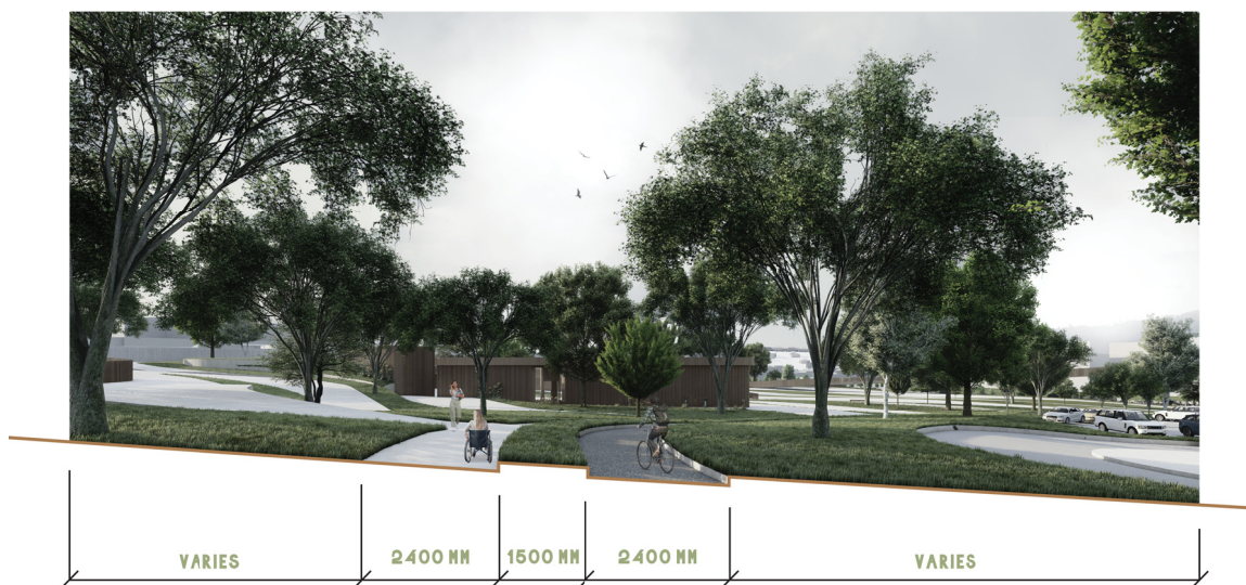
Diagram illustrates new bike and pedestrian paths integrated within the urban public landscape.
