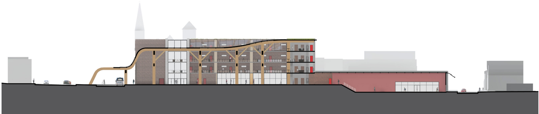
Section through the Red Block from Coldwater Road (left) to Mississauga Street (right), showing the bus stop, indoor market, public galleries, and arcade.
