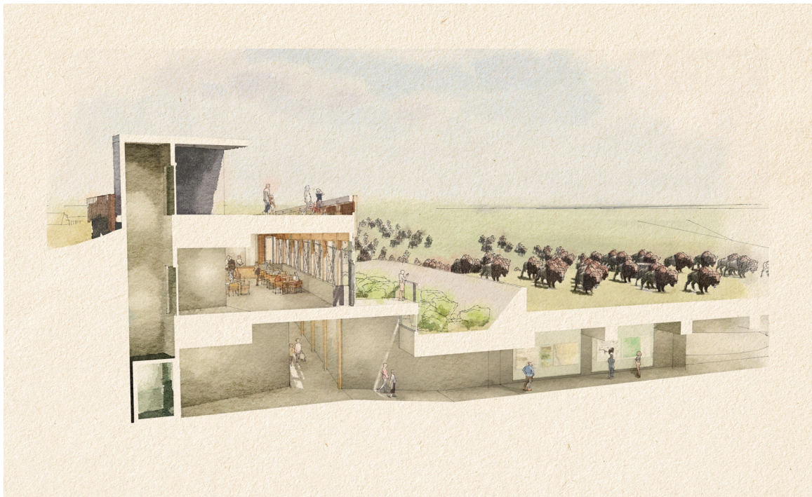
Figure 40. Section A - Showing the cafe and viewing dock that runs parallel to the land bridge. Underneath this bridge is a gallery hall that is centered by a reflection space in the middle of the facility.
