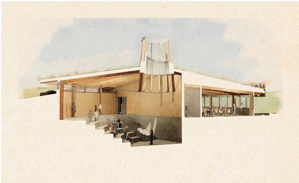
Figure 63. Section H: Section through the auditorium designed in a semi-circle to encourage discussion and the sharing of stories.
