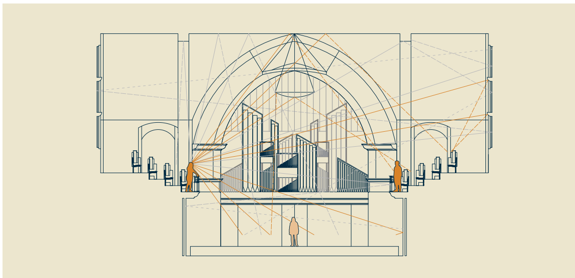
Lateral section, sound sources in side balconies 1:300
