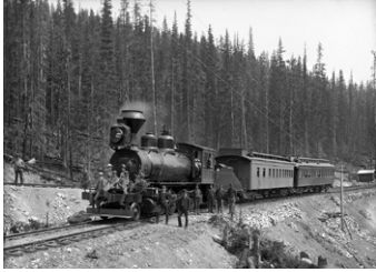
100-ton mountain engine on the Canadian Pacific Railway, BC, 1889; photographed by William Notman (Willis 2018)
