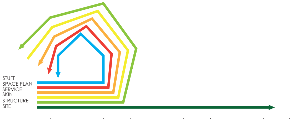
Unfolding the six layers of shearing layers diagram (base diagram from Brand 1995, 38)
