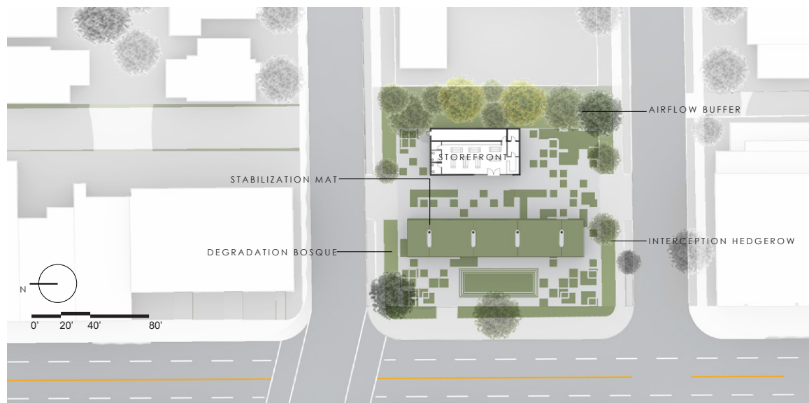
Plans for phase 1 that indicates where and what phytoremediation techniques are used on site.
