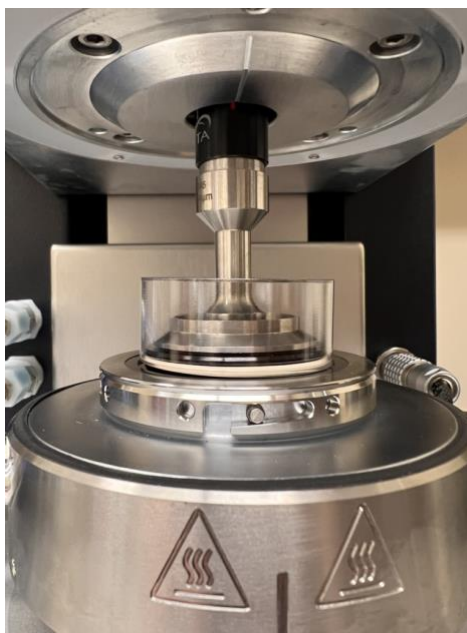
Figure 22: The HR 10 Discovery Hybrid Rheometer with cone and plate attachment. The device below the testing area is a warming plate used to control the temperature during the experiment.
