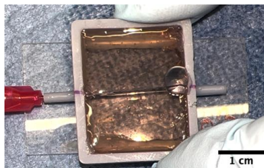
Figure 11: Optimization of the printing chamber geometry. The red syringe tip is inserted into the left side of the channel pushing water from left to right. Fluid buildup on the right side of the channel caused pooling of liquid on the surface of the matrix phase.
