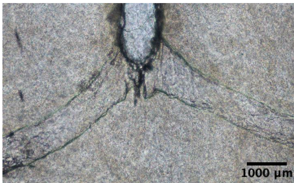
Figure 21: The result of an experiment where a channel was printed perpendicularly off a previously printed channel.
