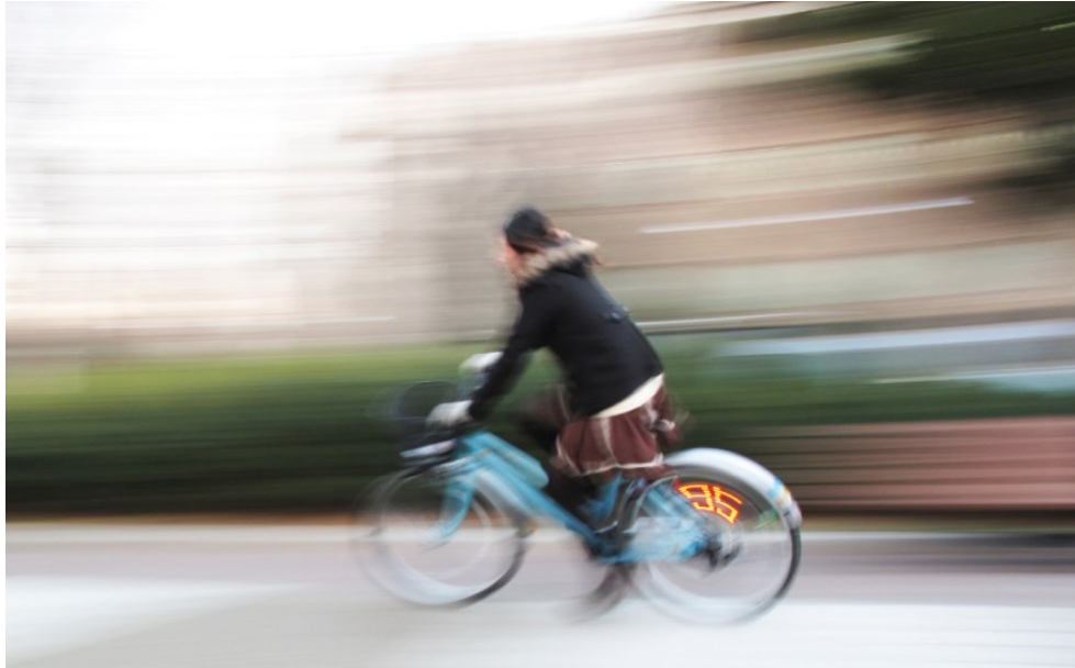
Figure 20 - AwareCycle (Kadomura et al., 2014) presenting the rider's heart rate on the rear wheel
