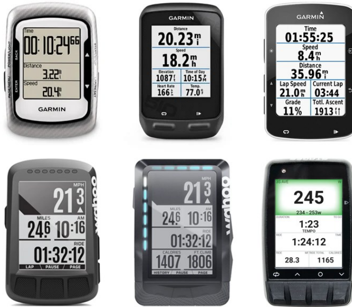
Figure 14 - Personalized data fields for several models of head units. Although units are from different manufacturers (Garmin, Wahoo, and Stages), their layout is similar. Source:
