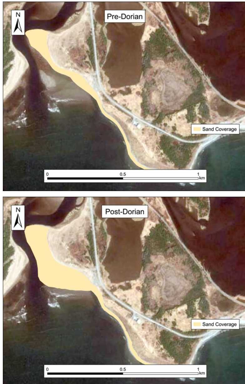
Figure D17 Aerial imagery map displaying sand coverage of Stoney (Lawrencetown) Beach in Halifax Regional Municipality, Nova Scotia, 1:5,000. Pre-Dorian photo: April 25, 2019; post-Dorian photo: April 18, 2020. There was a shifting of sand to create a sandbar within one-year following Hurricane Dorian from storm surge waves. Imagery was obtained with Google Earth Pro and ESRI World Imagery Wayback (Google, 2022).
