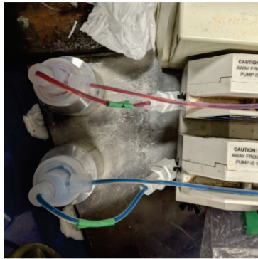
Charged 1x:negolyte (MEEV) is blue/green, posolyte (MEEPT) is red
