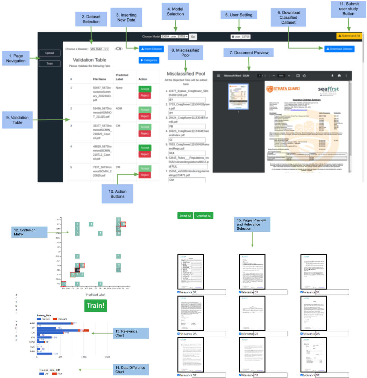
Figure 3.8: Frontend Screen Shots: The figure shows the screenshot from the user interface of the flask application used to take feedback from the user. The first image depicts the upload page and document annotation system, whereas the second image corresponds to the training page where the user can train the model and annotate the pages
