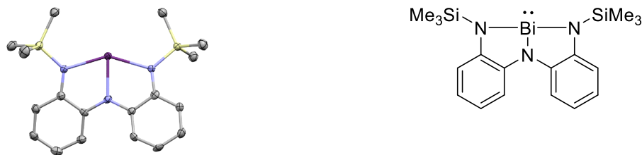
Figure 21. XRD-determined structure (left) and Lewis structure (right) of the N_3TMS_2 Bi compound made by the Chitnis lab, showing its planarity. Hydrogen atoms omitted for clarity.
