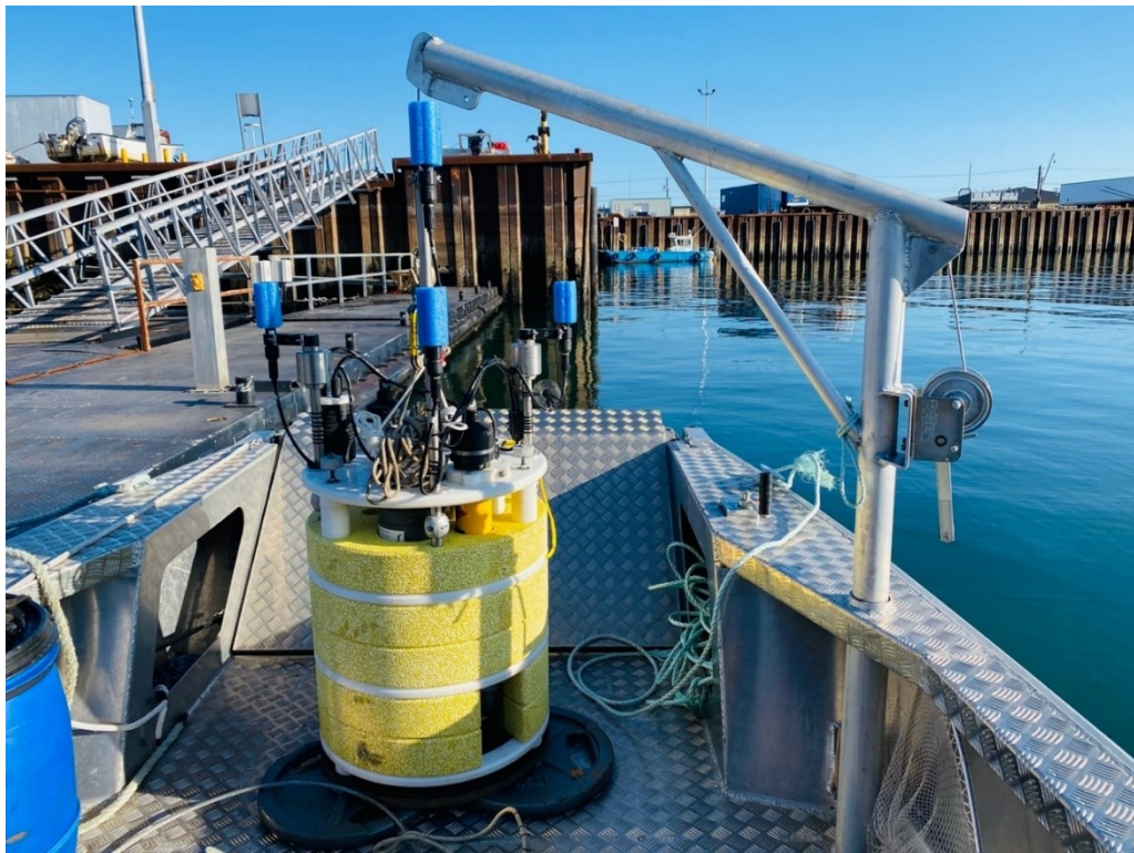
Figure 9: JASCO AMAR integrated on C-Lander mooring.
