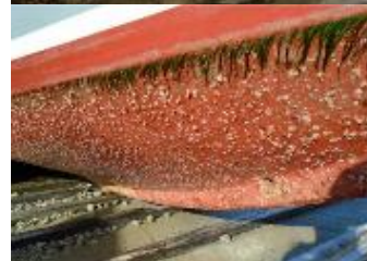
Figure 46: Photos of Charlie and Delta after a season of summer fouling growth.
