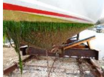
Figure 45: Photos of Alpha and Bravo after a season of summer fouling growth.
