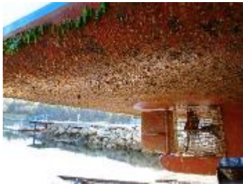
Figure 45: Photos of Alpha and Bravo after a season of summer fouling growth.
