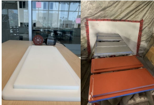
Figure 16: HDPE panels after surface preparation and coating application
