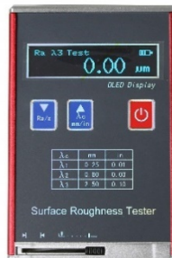
Figure 17: VTSYIQI surface roughness gauge used for panel roughness measurements (Ra, Rz, Rq, Rt).
