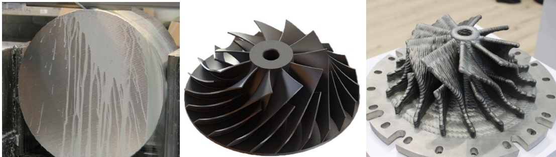
Figure 27: Traditional cylindrical stock (left) compared to near-net-shape additively manufactured stock (right) and the resultant machined part (center) [78].
