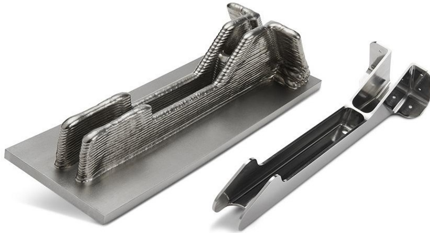
Figure 30: Deposited near-net-shape stock (left) and final machined part (right) [93].
