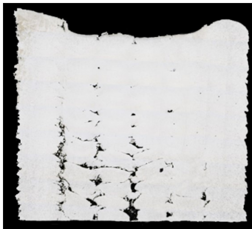
Figure 60: Porosity induced in a build of Beta-21S due to excessive hatch spacing. Sample fabricated with a hatch spacing of 2.67 mm.
