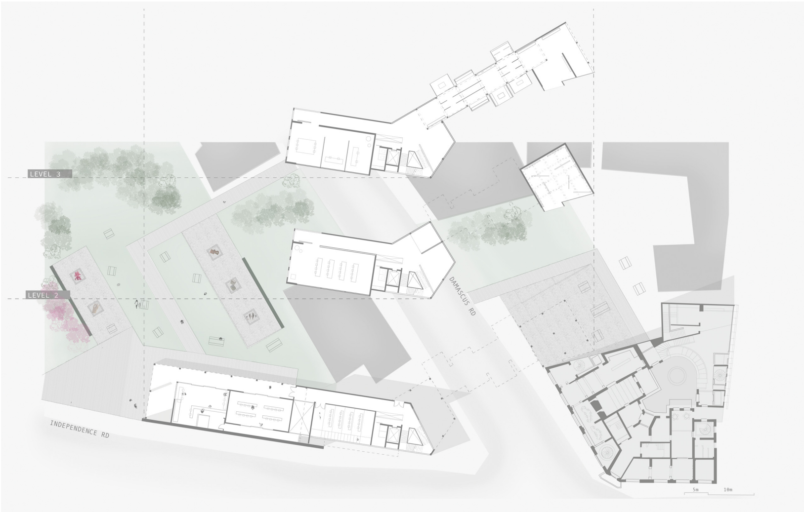
Figure 47: A breakdown of the site and building extension in relation to Beit Beirut. There are three levels to the addition, ground level, second level in the middle of the image, and third level towards the top that encompasses a bridge, connecting both parts of the addition together and towards the third level of the museum.
