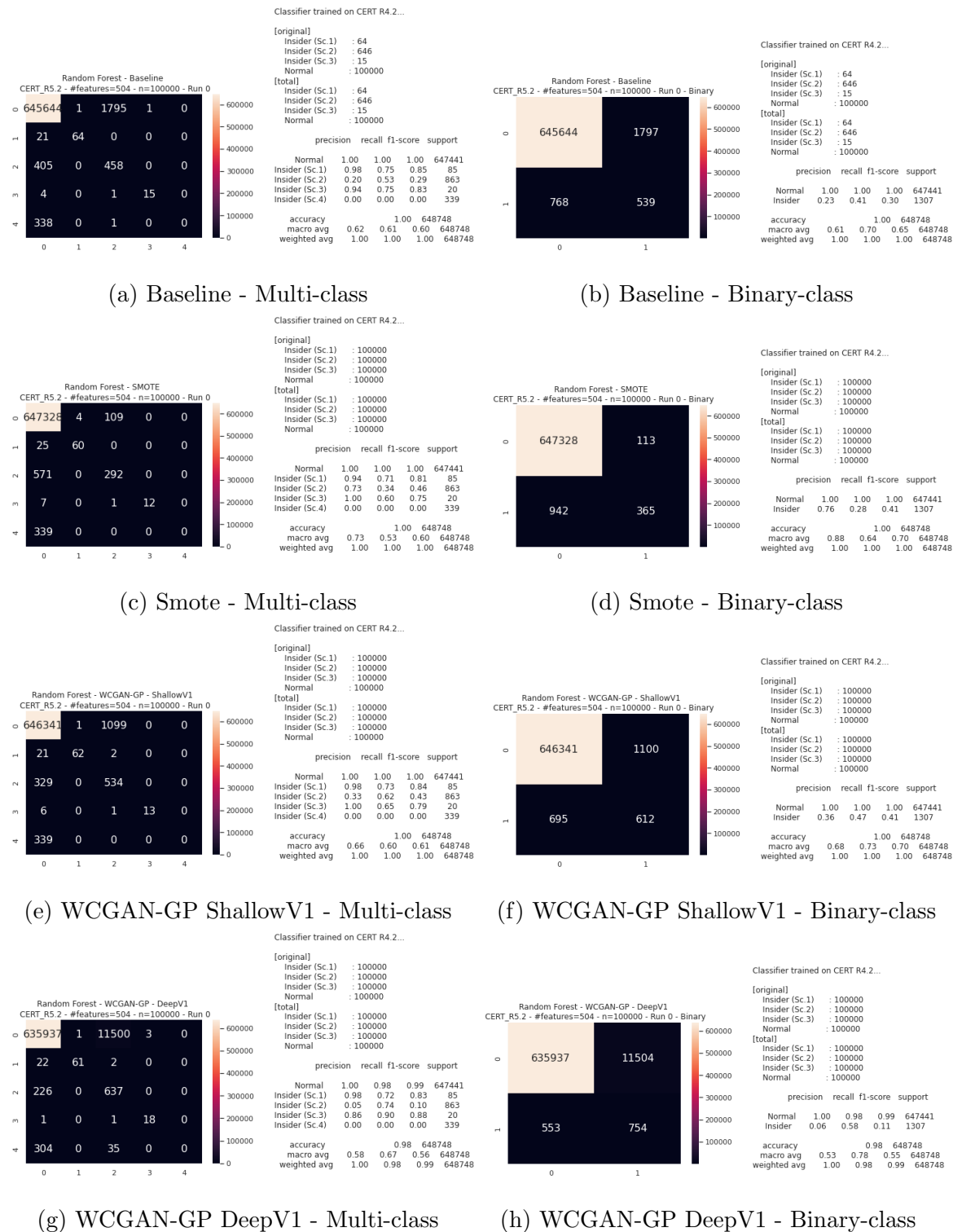
Figure A.4: CERT R5.2, 504 features: Sample confusion matrices for random forest classification
