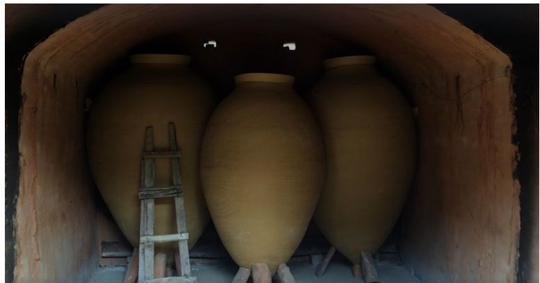
Qvevri in the kiln (Railsback 2018).
