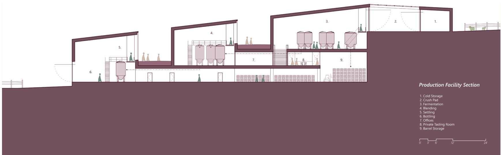
Production facility section.
