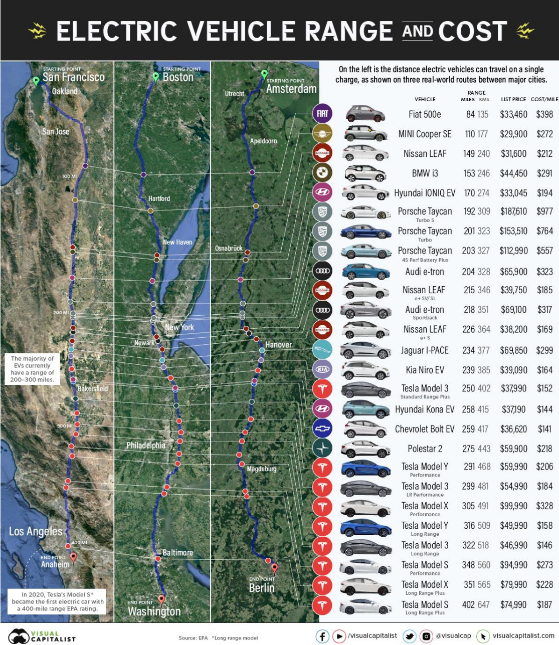
Figure 1.1 | Electric vehicle range. List of electric vehicle models and their range and price as of September 2020. The ranges are ranked and visualized depicting possible journeys over three different routes. This graphic was produced by Visual Capitalist: https://www.visualcapitalist.com/range-evs-major-highway-routes/
