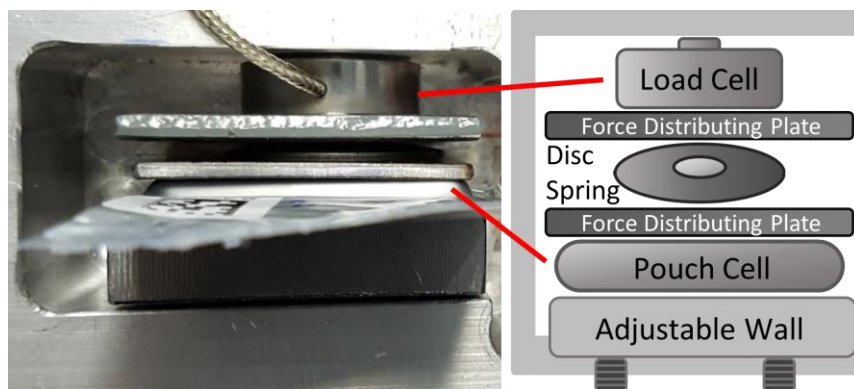
Figure 3.4 | Superboat pressure measurement. Picture (left) and schematic representation (right) of the superboat cell testing setup. Pouch cells are fastened by an adjustable wall which can be tightened to change the pressure and a load cell used to measure the pressure, separated by force distributing plates and a disc spring.
