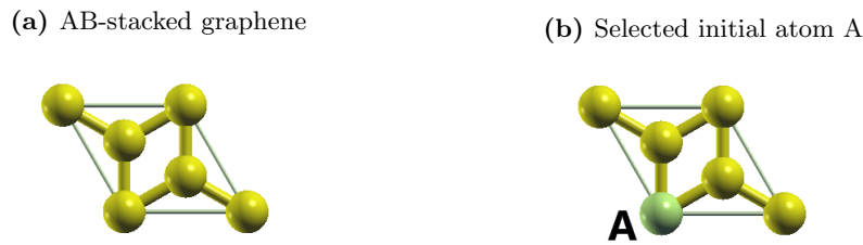
Figure 3.1: 1 \times 1 AB-stacked structure of bilayer graphene showing the selected initial atom.
