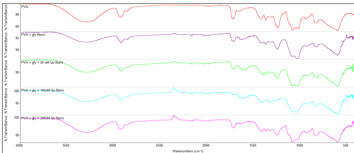
Figure 18 IR spectra for PVA fibers loaded with quercetin.
