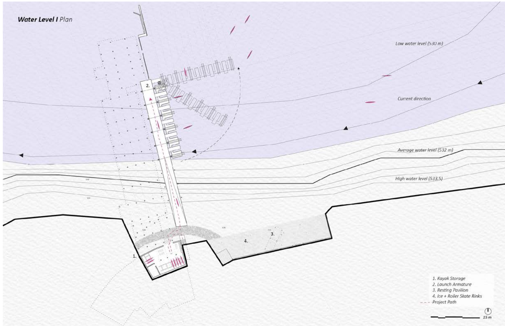
Water level. Plan of the kayak storage and launch armature showcasing the armature's ability to rotate with the seasonal fluctuations.
