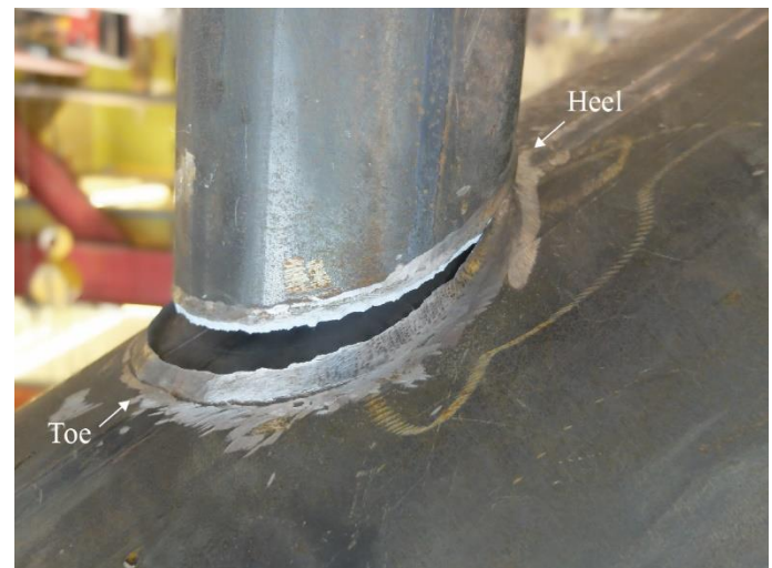
Figure 5. Weld fracture in test 102-406-60a
