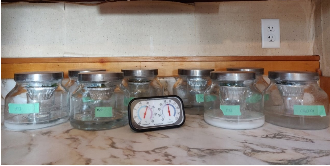
Figure 14 Glass jars used for static gravimetric method (by Challa).
