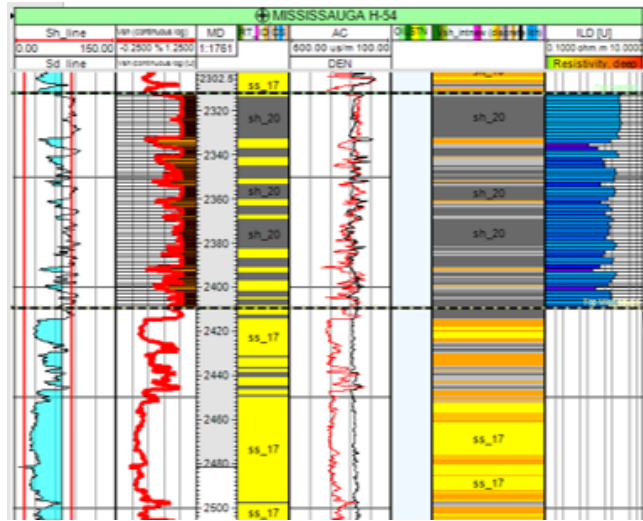
Figure 5.12: Log sample from the Mississauga H-54 well through a section showing the Naskapi Member. The unit is bounded by black dashed lines and combines wireline logs (from left to right): gamma ray, sonic, density and deep resistivity) with lithologs that clearly highlight the yellow sand and grey shale intervals.
