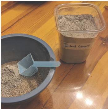
3 - Mix the filtered earth with filtered sand and Portland cement (80% earth, 10% sand & 10% cement).
