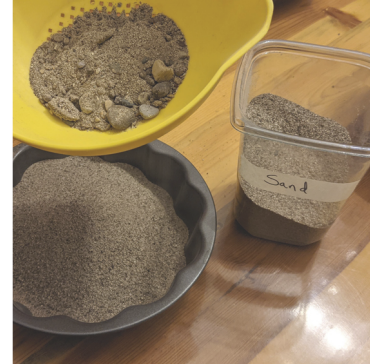
2 - Filter the sand to remove rocks.
