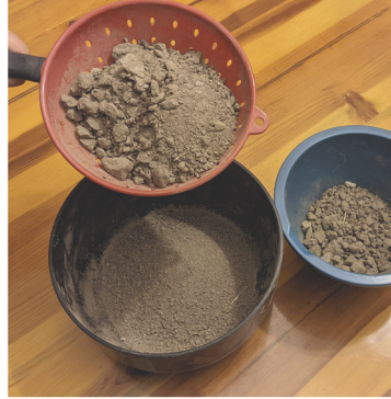
1 - Filter the earth to remove rocks and waste.
