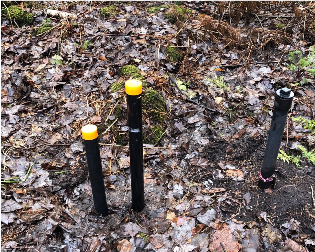
Figure 4: Piezometer nests in Cornwallis River Treed Swamp installed on December 5, 2019
