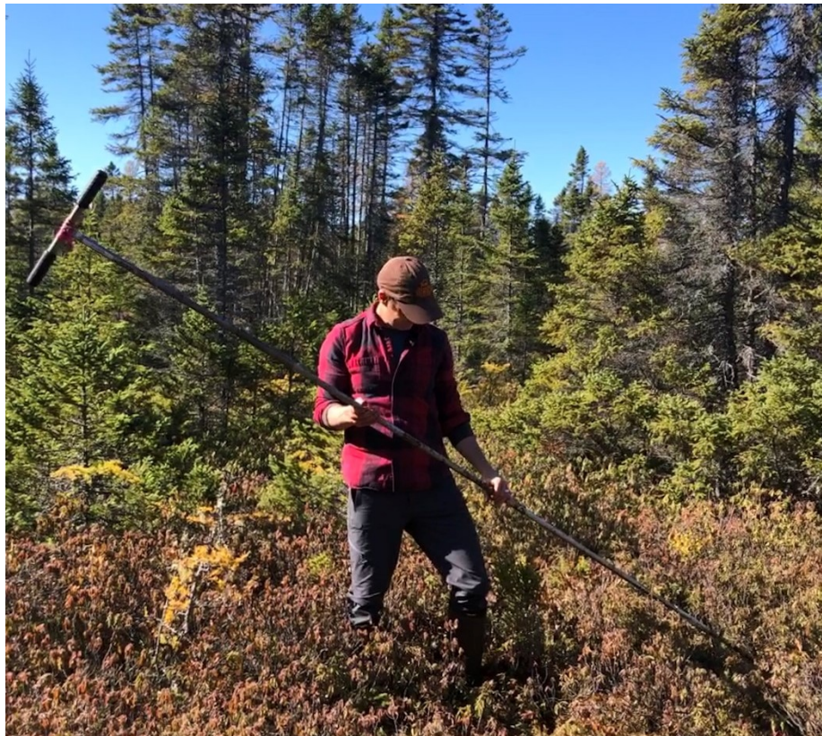
Figure 6: Auger used to drill boreholes for peat decomposition testing.
